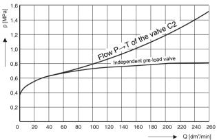
Maximal flow through pre-load valve 260dm<sup>3</sup>/min.
