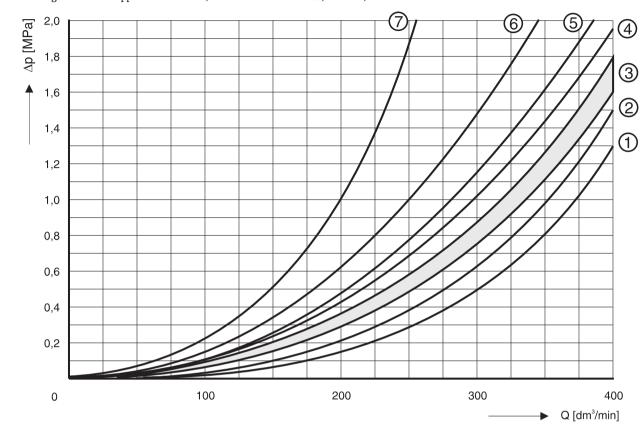
**Note:** average values with upper deviation 20%, measured at  $v = 35 \text{ mm}^2/\text{s}$ , T = 50°C,
