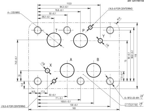
Description of ports: P ..... input of pressured oil into the main valve
