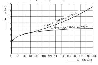
Maximal flow through a pre-load valve 260 dm<sup>3</sup>/min.
