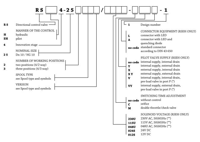
(\*) Spool types: C1, C2, L1, L2 (\*\*) Connector with rectifier
