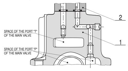
External pilot oil supply and drain Operating time is controlled by a flow orifice.
