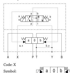
Internal pilot oil supply (X), external pilot oil drain (Y)
